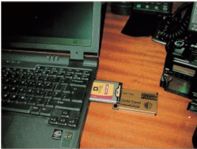
Fig. 2 PCMCIA card slots into the laptop.
